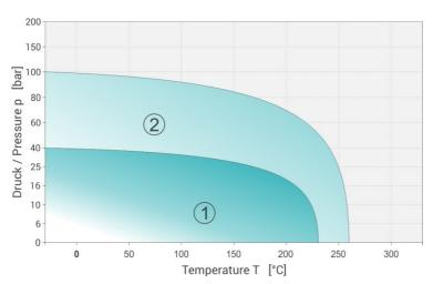
The p-T diagram indicates the service limits considering the simultaneous influence of pressure and temperature.
